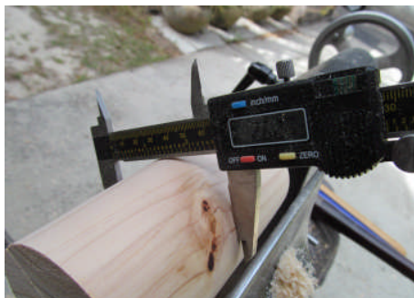
Using a Vernier, dial or digital caliper, measure the diameter of the cylinder.
