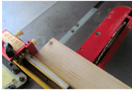
Cross-cut the length to equal: Width + 2"
