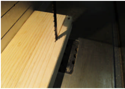
Rip width to equal two thicknesses of the planed stock.
