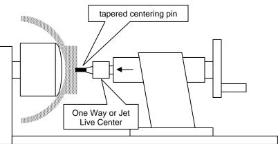
Using Geiger's Re-Centering Solution with a face plate.
