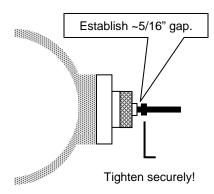
Note: The gap can vary depending on the amount of waste stock that remains at the bottom of your work piece. Just make sure that there is enough to make a hole deep enough so the centering pin will hold securely, but not so deep that you go through the bottom of your piece.
