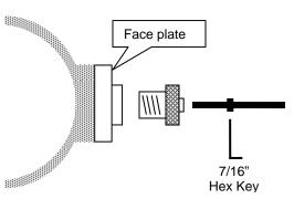
Locate the Re-Centering device, drill bit, stop collar and hex key. Test to ensure that the drill bit fits through the drill bushing.
