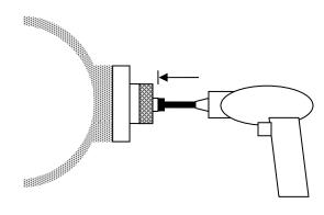
Position the work piece against a jam chuck or vacuum chuck. Slide the tail stock forward until the centering pin goes into the previously drilled hole. Secure the tail stock. Advance the tail stock quill until enough
